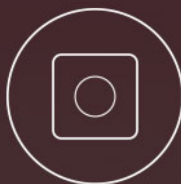
On/Off, Dimmer (Wall) Switch
